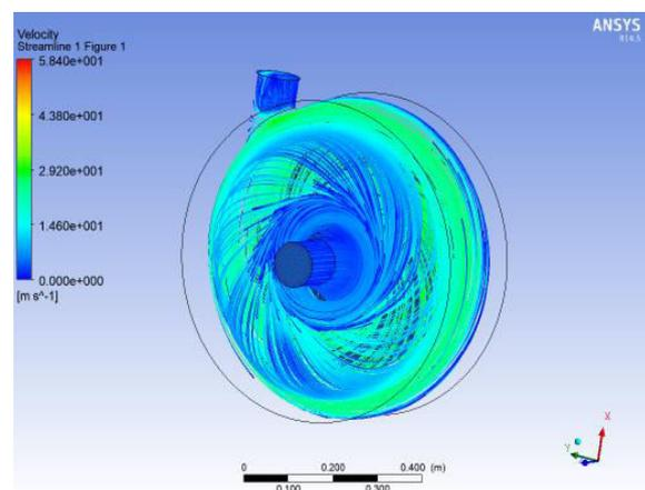
A Manivannan. "Computational fluid dynamics analysis of a mixed flow pump impeller" International Journal of Engineering, Science and Technology Vol. 2, No. 6, 2010, pp. 200-206.
