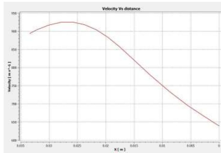
Fig. 6. Velocity versus distance along the nozzle.
