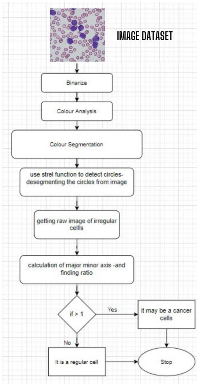
Figure 2. Flowchart of the developed classification system
