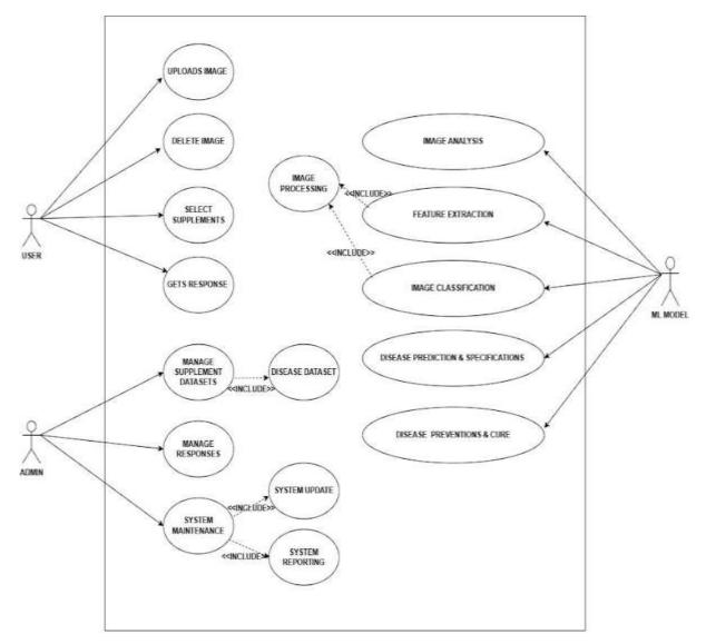
Fig. Use Case Diagram of Computer Vision Plant Diagnostics
