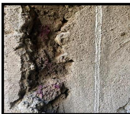
**Figure 5 Phenolphthalein solutions on concrete surface**
