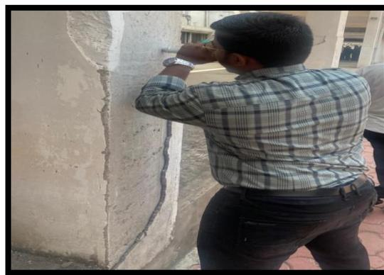
**Figure 12: Process of using Rebound Hammer**
