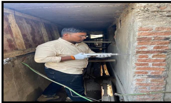
Figure 3: Process of using Rebound hammer
