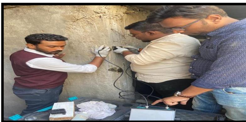
**Figure 4: Process of using Ultrasonic pulse velocity test**
