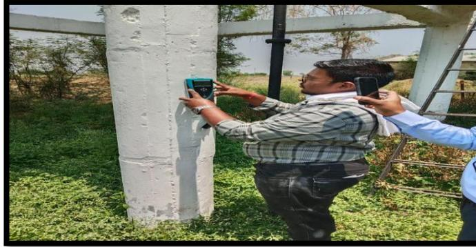
**Figure 20: Rebar locator**
