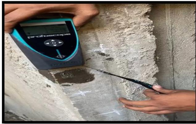
**Figure 6: Position of reinforcement in the column**
