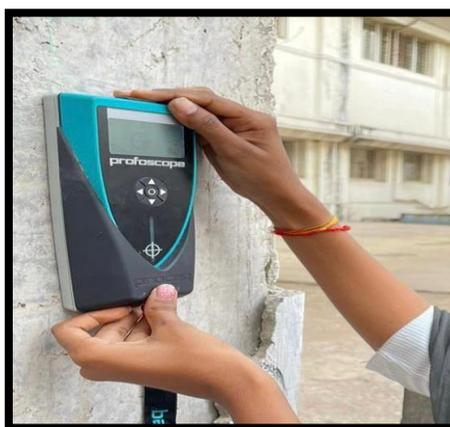
**Figure 14: Position of reinforcement in the column**
