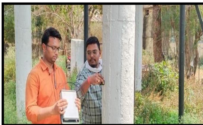
Figure 19: Ultra sonic pulse velocity test
