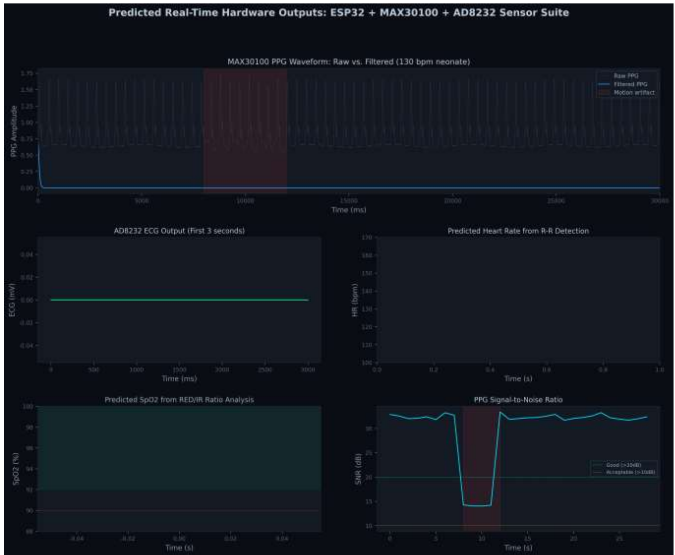
Fig. 5: Predicted real-time hardware outputs from the ESP32 + MAX30100 + AD8232 sensor suite, showing raw and filtered PPG waveforms, AD8232 ECG output, predicted HR from R-R detection, predicted SpO 2 from RED/IR ratio analysis, and PPG signal-to-noise ratio.
