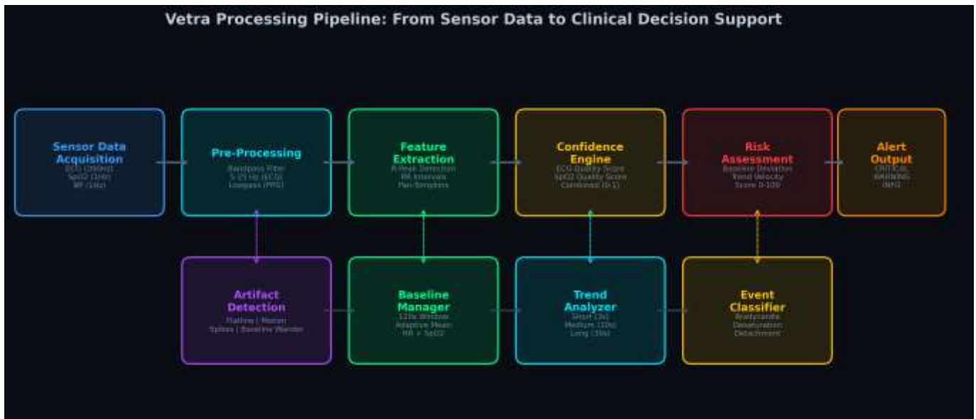
Fig. 2: Vetra software processing pipeline: raw sensor data flows through pre-processing, feature extraction, confidence assessment, and risk scoring before generating clinical alerts. Parallel processes handle artifact detection, baseline management, and trend analysis.
