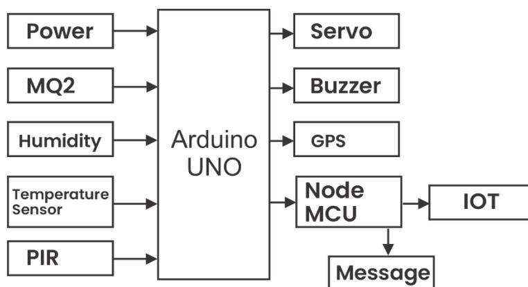
The initial phase of this project involves the creation of an alarm circuit to be integrated into the prototype. Once the receiver circuit identifies the presence of gas leakage, it transmits signals to the relay circuit. Consequently, the alarm system is automatically triggered to alert users of the potential gas leakage.
