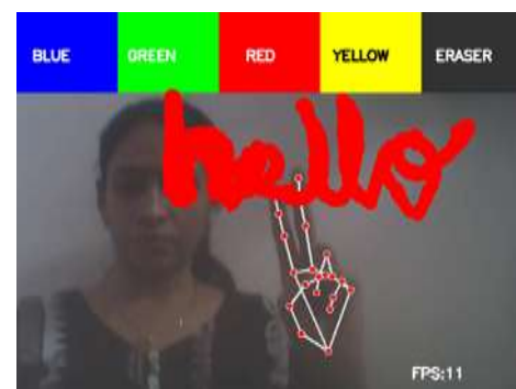
Fig- 3. Drawing output without the LSTM filter (FPS: 11).
