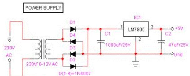
Figure 3. Circuit diagram of power supply system.
