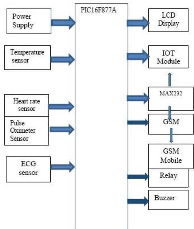
Figure 2. Architecture of health monitoring system based on IoT.
