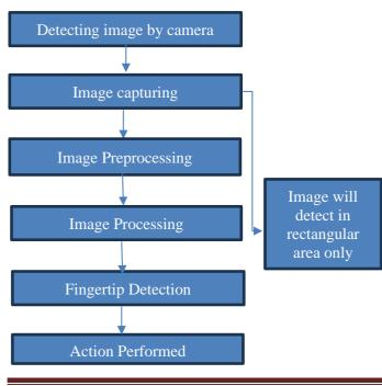
**1.** Detecting image by camera: The camera or webcam takes the user's hand's real-time image or video feed. The camera is essential for generating visual data, which forms the foundation for gesture detection.
