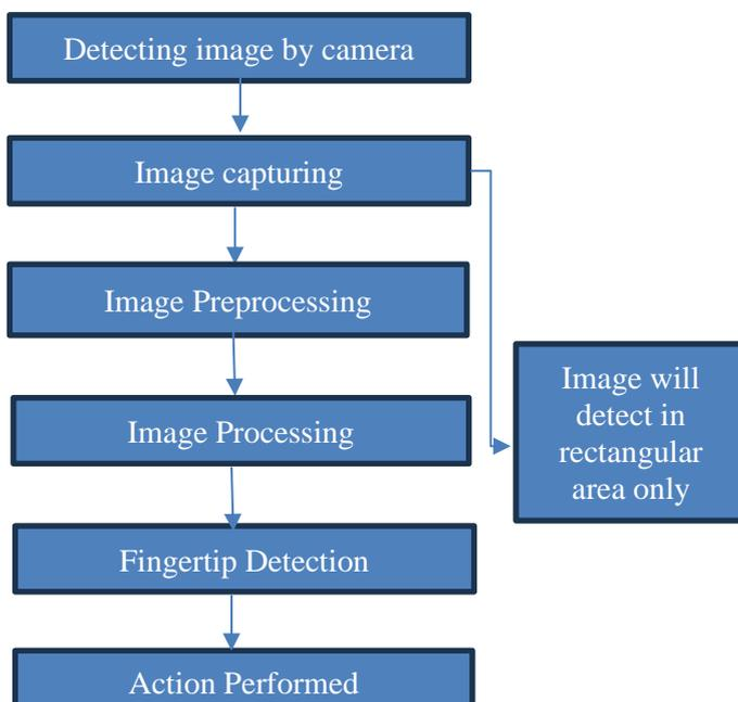
**1. Detecting image by camera:** The camera or webcam takes the user's hand's real-time image or video feed. The camera is essential for generating visual data, which forms the foundation for gesture detection.
