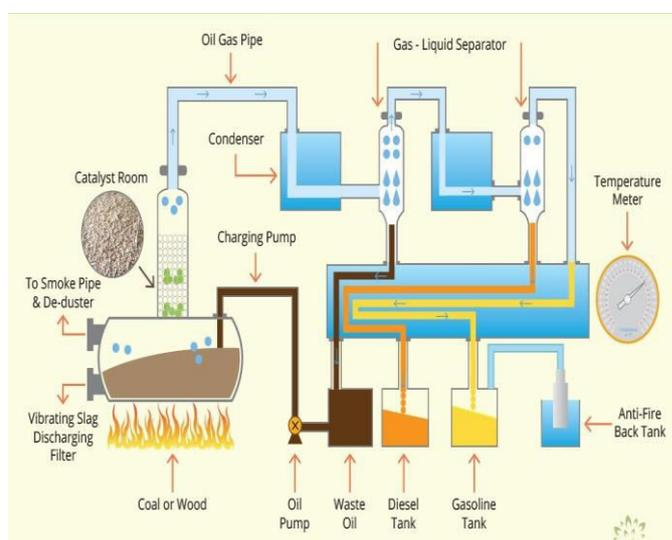
Fig -1: Plastic Pyrolysis Process
