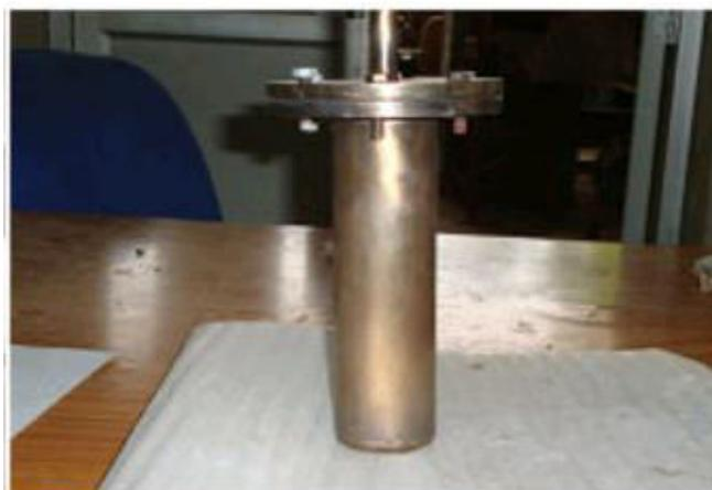
Fig-2: Stainless steel Reactor
