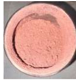
Figure 4. Graphite Powder mixed with Copper powder and PEG
