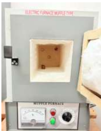
Figure 7. Sintering of specimen in electric furnace muffle type
