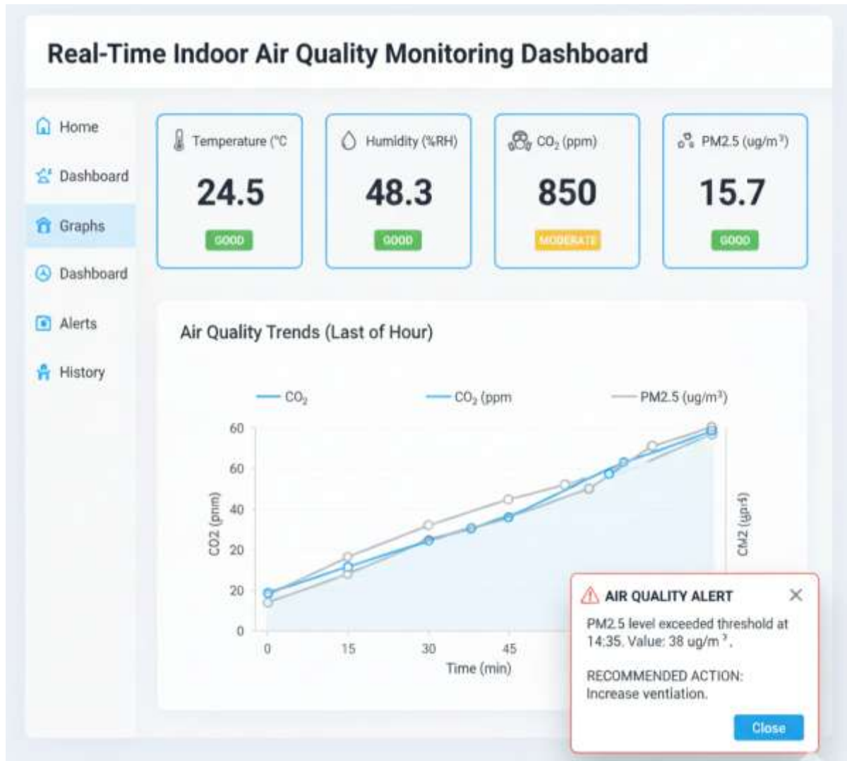
Figure 5: Cloud dashboard interface showing real-time visualization of IAQ parameters and alert status
