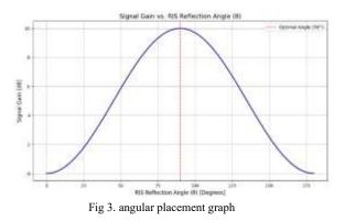
The graph confirms that **even minor misalignments from the optimal 90° orientation lead to a steep drop in gain**, which reinforces the importance of precise angular placement in real-world deployments. This finding is implemented in the MATLAB simulations of this project, where RIS panels are positioned at a ~120° spread around a central building to maximize coverage in Non-Line-of-Sight (NLOS) regions.
