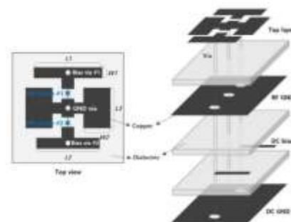
Fig. 1. Structural design of a reconfigurable intelligent surface (RIS) unit cell, illustrating the layered architecture with PIN diodes, vias, and biasing structure.
