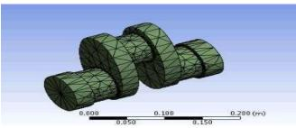
I have chosen tetrahedral mesh because the tetrahedral meshing methodology is utilized strong district geometry cross section and meshing delivers a good support for boundaryrepresentation of solid auxiliary model.
