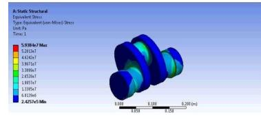
The Material which was maximum deformation is found to be Structural Steel. In the case of Equivalent Strain, the material which has least maximum value is structural steel. Finally, the material which has least maximum value for
