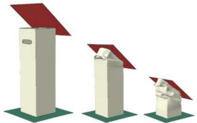
Fig -12: Deformation sequence of the two-hole tube under oblique crushing ( 45^\circ ).
