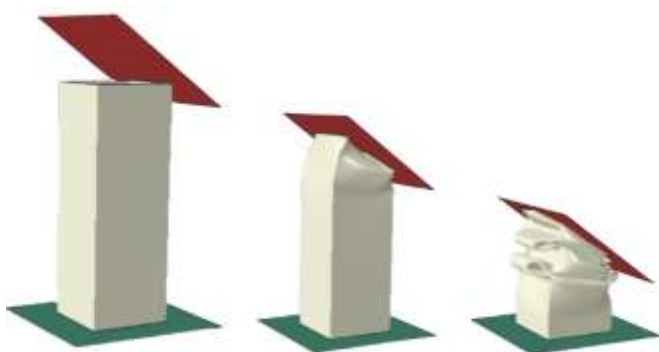
Fig -11: Deformation sequence of the intact tube under oblique crushing ( 45^\circ ).
