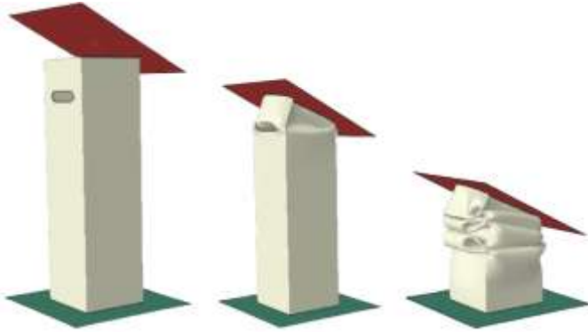
Fig -8: Deformation sequence of the two-hole tube under oblique crushing ( 30^\circ ).
