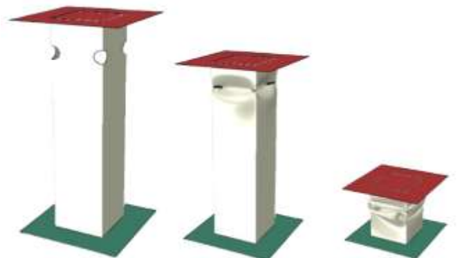
Fig -5: Deformation sequence of the elliptical-hole tube under axial crushing (0°).
