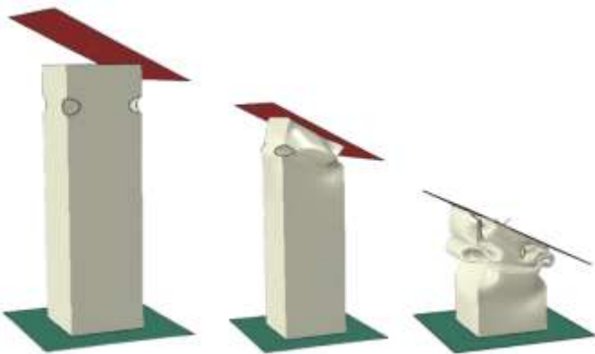
Fig -9: Deformation sequence of the elliptical-hole tube under oblique crushing ( 30^\circ ).
