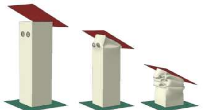
Fig -7: Deformation sequence of the intact tube under oblique crushing (30°).
