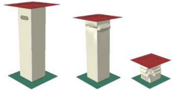
Fig -5: Deformation sequence of the elliptical-hole tube under axial crushing (0°).
