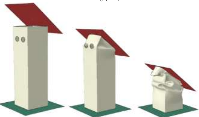
Fig -11: Deformation sequence of the intact tube under oblique crushing ( 45^\circ ).
