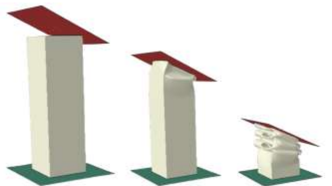
Fig -7: Deformation sequence of the intact tube under oblique crushing (30°).
