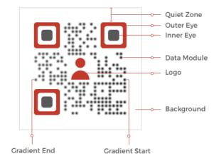
Fig 4. Basic structure of QR Code
