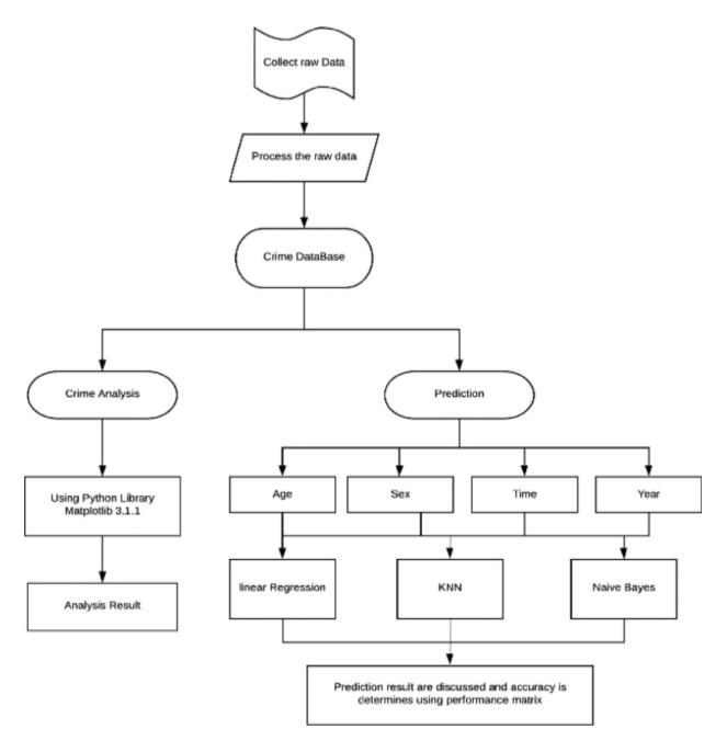
The Crime Data Analysis System (CDAS) is designed as a comprehensive solution for law enforcement agencies and policymakers, integrating various stages from data collection to real-time analysis. It starts with gathering and preprocessing diverse data sources, ensuring cleanliness and relevance for subsequent analysis. Feature selection is crucial, incorporating key factors like location, time, crime type, and socio-economic indicators to provide
