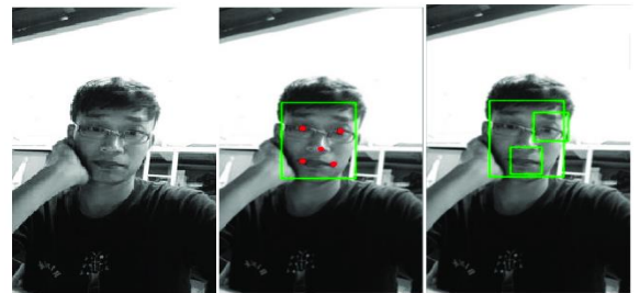
Fig3.3.2: By using Multi-Task Cascaded Convolution Network Algorithm
