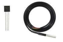
DS18B20 temperature sensor in all fairness particular and wishes no outside additives to paintings. It can be degree temperatures from -55 °C to +125 °C with  $\pm 0.5$  °C Accuracy. The decision of the temperature sensor is user-configurable to 9, 10, 11, or 12 bits. However, the default decision at energy-up is 12-bit (i.e. 0.0625 °C precision). The sensor may be powered with a 3V to 5.5V energy deliver and consumes handiest 1mA at some point of energetic temperature conversions.
