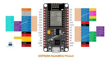
The ESP8266 is a low-cost Wi-Fi microchip with full TCP/IP stack capabilities, widely used in IoT applications. Developed by Espressif Systems, this module allows devices to connect to Wi-Fi networks and transmit data over the internet, making it ideal for smart home devices, remote sensors, and other IoT projects.
