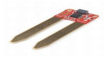
A soil moisture sensor is used to detect the amount of water present in the soil. Unlike traditional gravimetric methods, which require removing, drying, and weighing a soil sample, these sensors determine water content indirectly. They do this by analyzing soil properties that shift with moisture, such as dielectric constant, electrical resistance, or neutron interaction, which correspond with soil water levels.
