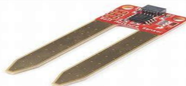
A soil moisture sensor is used to detect the amount of water present in the soil. Unlike traditional gravimetric methods, which require removing, drying, and weighing a soil sample, these sensors determine water content indirectly. They do this by analyzing soil properties that shift with moisture, such as dielectric constant, electrical resistance, or neutron interaction, which correspond with soil water levels.
