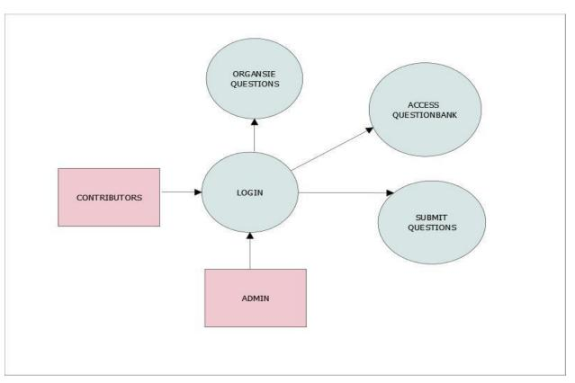
Figure 2.2. Level 1 Data Flow Diagram
