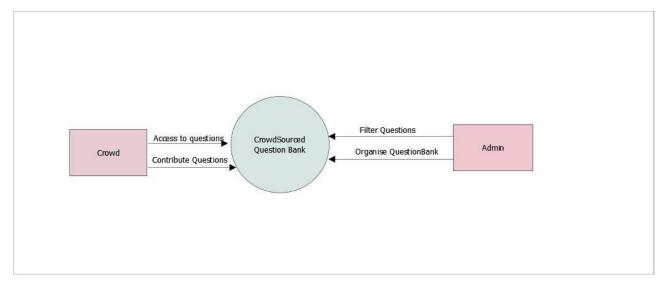
Figure 2.1. Level 0 Data Flow Diagram
