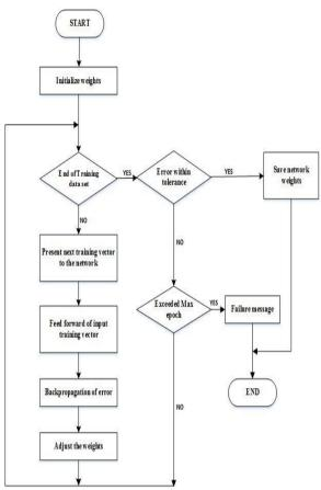
Fig.3 Flowchart of Back Propagation
