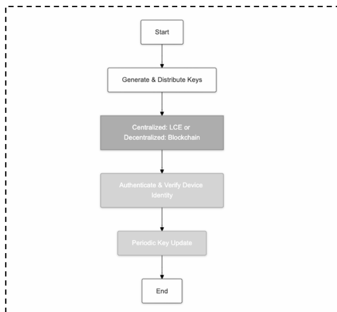
Flowchart for key distribution and management in IoT, covering both centralized and decentralized approaches
