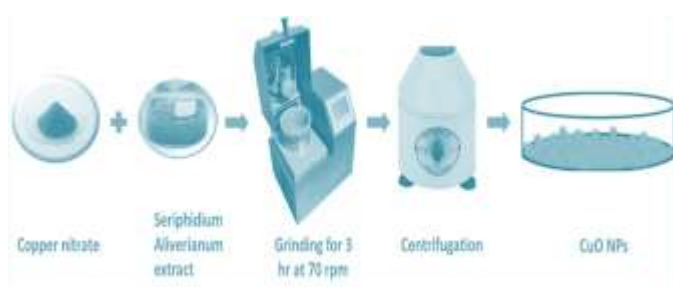
Fig 7. Synthesis of CuO-NPs by mechanochemical methods and sources of biogenic copper oxide nanoparticles.
