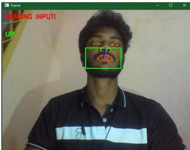
**Fig No: 7. Detecting Eye movement in the upper direction**
