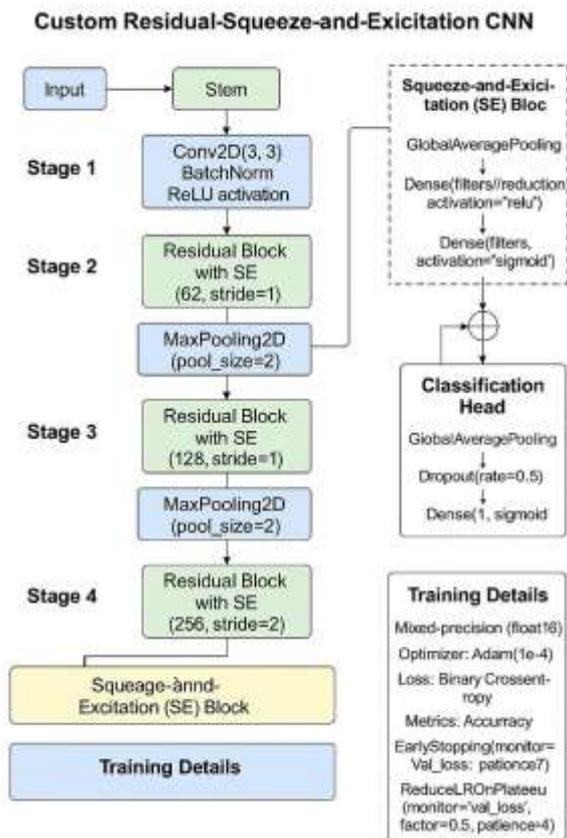
Fig. 3. Proposed Residual SE-CNN Architecture
