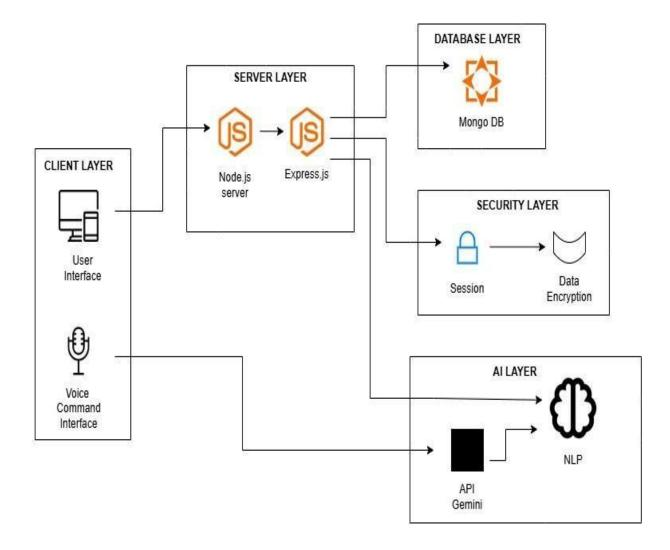
The system architecture for the chatbot can be visualized as a client-server model, where the client (user) interacts with the chatbot via a web interface or voice command, and the server handles requests, processes them, and returns responses. Below is the basic structure:
