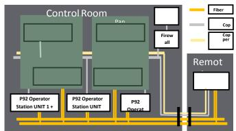
There are North (corporate network facing Firewalls) and South (Plant Network Facing Firewalls). Configuration is done for the security development of the Plant network as well as network device itself.
