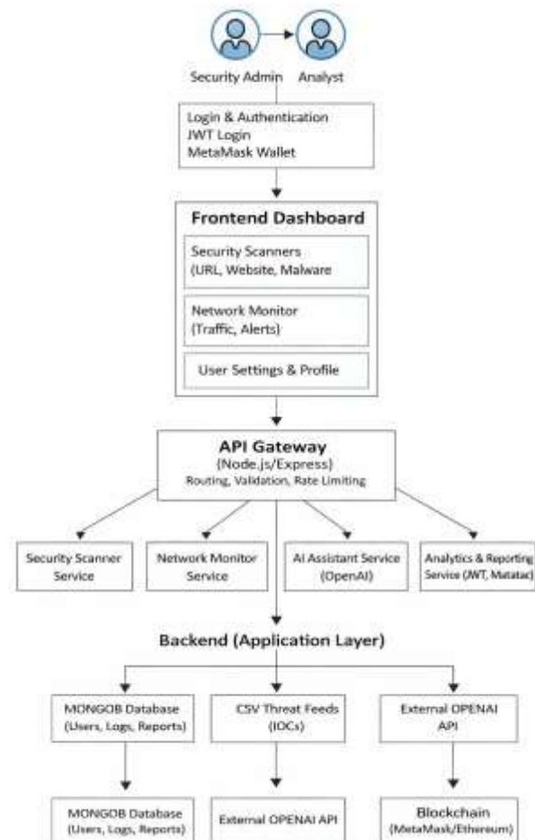
The CyberGuard AI platform follows a layered architecture designed to provide secure, scalable, and intelligent cybersecurity monitoring. At the user level, the system supports security administrators and analysts who access the platform through a web-based interface with secure authentication using JWT and blockchain-backed wallet verification.
