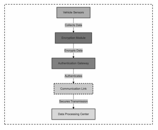
**Diagram**: Encrypted Communication Flow for Autonomous Vehicles, outlining secure data exchange pathways, including encryption and authentication checkpoints.
