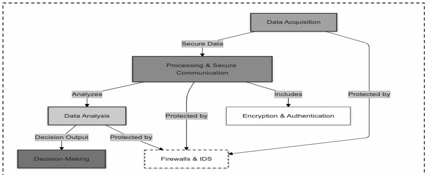
**Flowchart:** Autonomous System Cybersecurity Architecture, showing the layers of security measures from data acquisition to decision-making.
