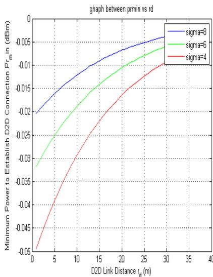
Fig. 6 Minimum Power Required to establish D2D link as a function of distance and fading (sigma)
