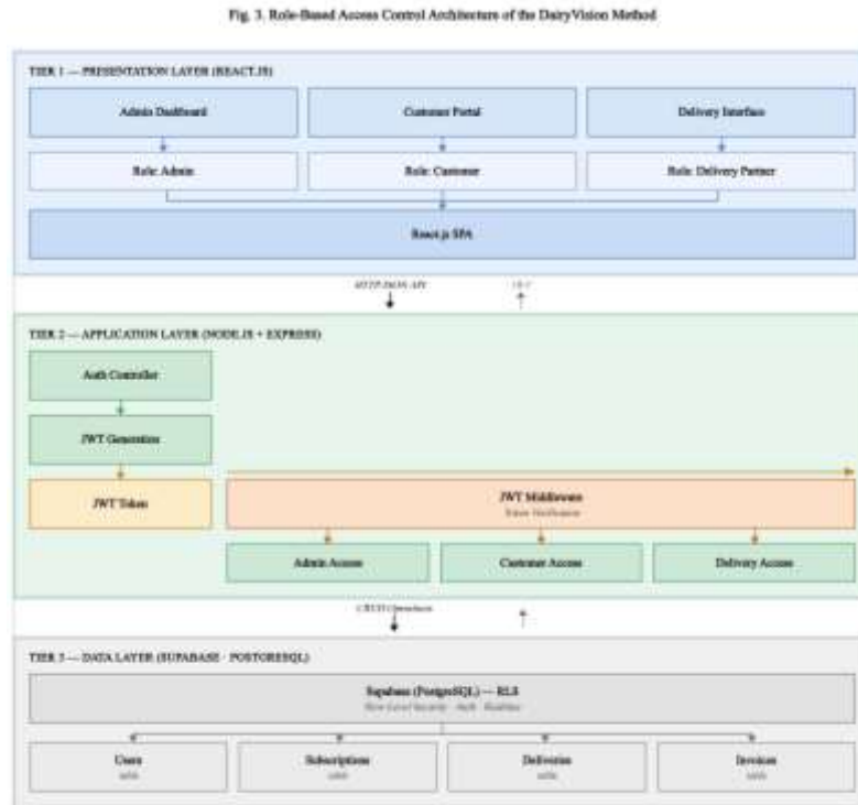
Fig. 3. Role-Based Access Control (RBAC) Architecture — JWT middleware validates role claims before routing requests to API endpoints.
