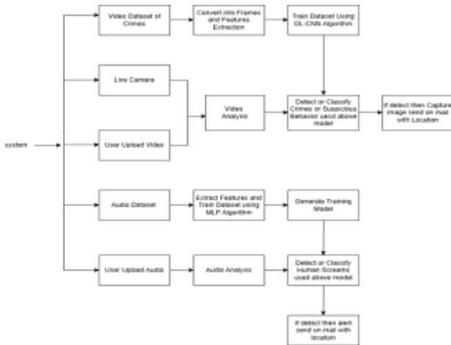
Fig. 1. System Architecture of Deep Learning-Based Suspicious Activity and Scream Detection System
