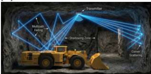
Figure 2: Radio Frequency Signal Propagation in Underground Tunnels
