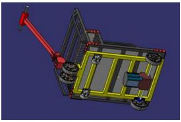
Fig. No.4 - Motors bogie frame
