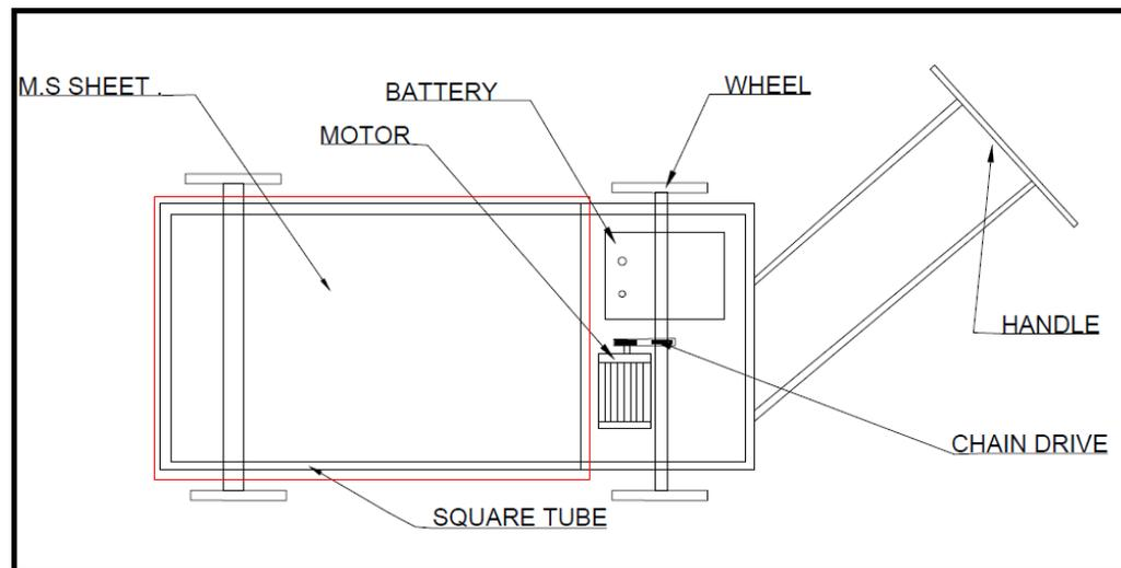
Fig. No.3 - Conceptual block diagram
