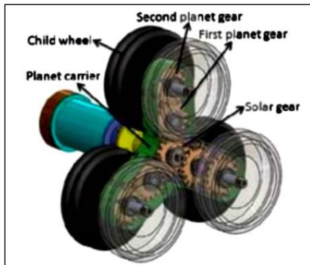
Fig. No.14 - Mechanism of Tri- Star Wheel
