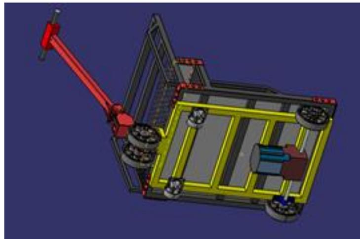
Fig. No.4 - Motors bogie frame
