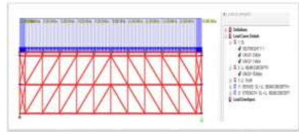
Figure No.03: Loading on Truss
