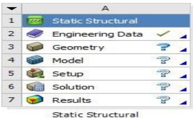
**The Static Structural Analysis (SSA) tab**
