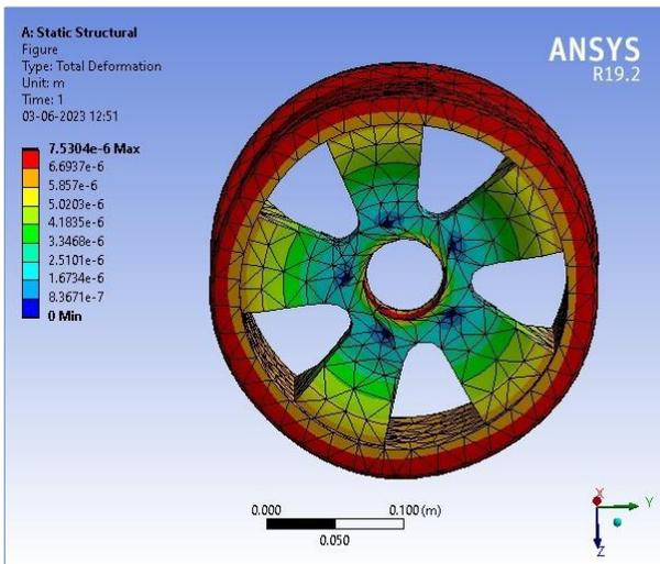
The Mini and Max Values of Total Deformation of an Alloy Wheel
