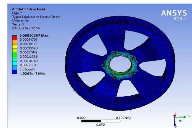
The Maxi and Mini Values of Equivalent Elastic Strain
