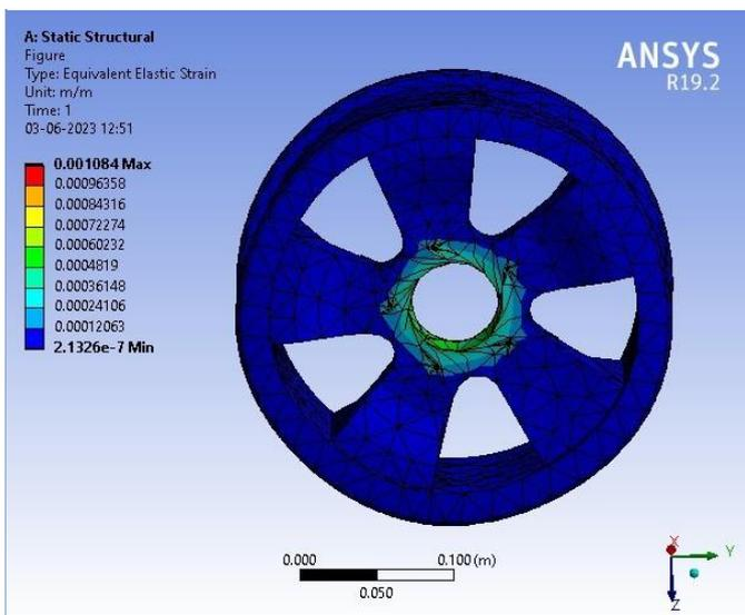
The Maxi and Mini Values of Equivalent Elastic Strain
