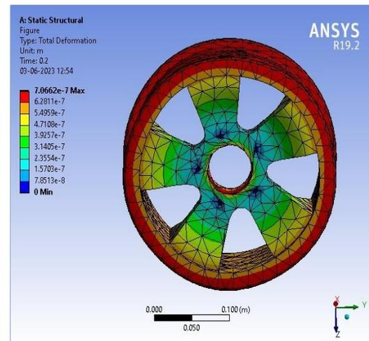
The Mini and Max Values of Total Deformation of an Alloy Wheel
