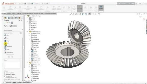
**Fig 2. Bevel gear design**
