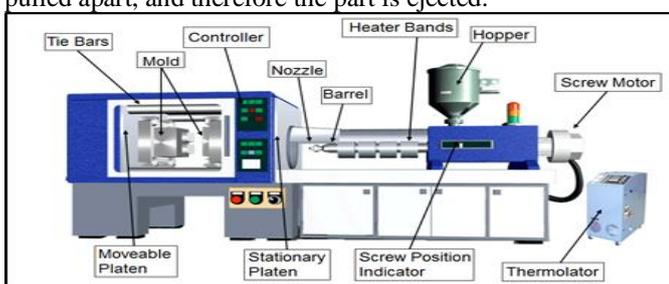
Figure 1: Injection Molding Machine
