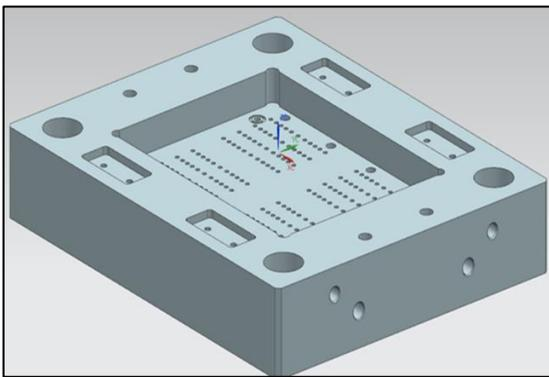
Figure 18: Core Housing Top view
