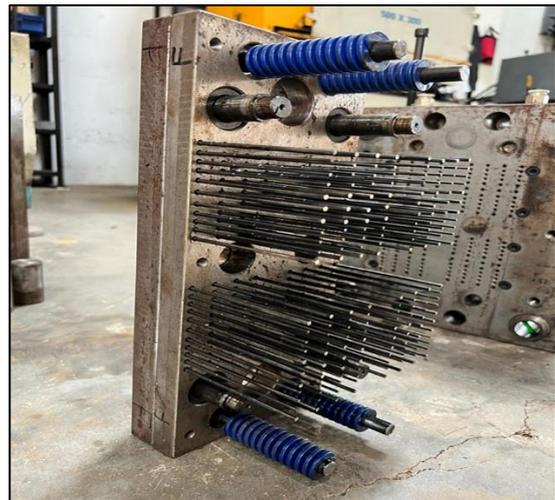
Photograph 28: Ejector Plate
