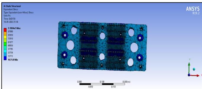
Figure 41: Stress induced in Ejector Plate
