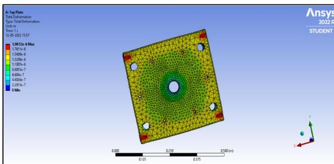
Figure 52: Total deformation of Top Plate
