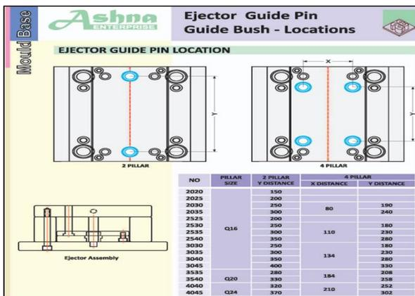
Figure 10: Standard Ejector Guide Pin and Guide Bush Locations
