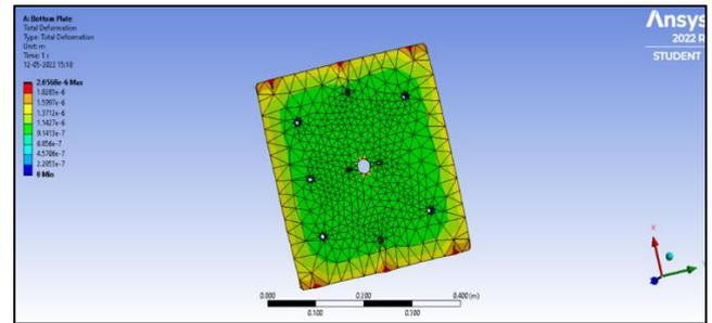
Figure 44: Total deformation of Bottom Plate
