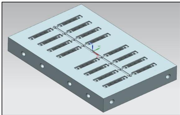
Figure 23: Core Block Top View
