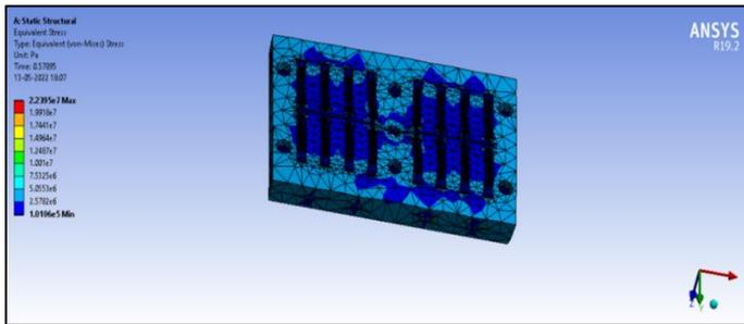
Figure 40: Equivalent stress induced in Cavity Block
