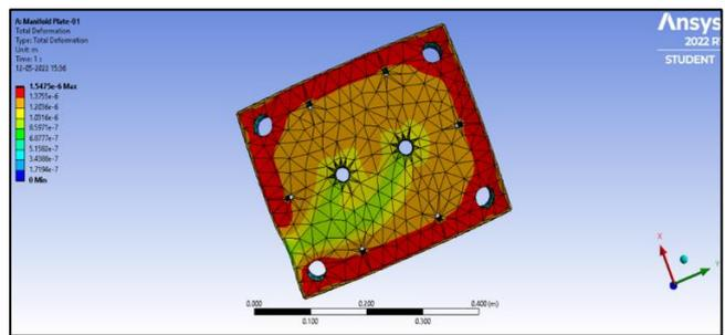
Figure 46: Total deformation of Nozzle Plate
