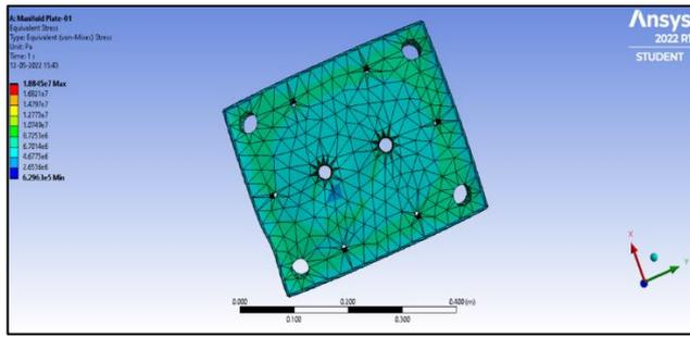
Figure 49: Stress induced in Nozzle Plate
