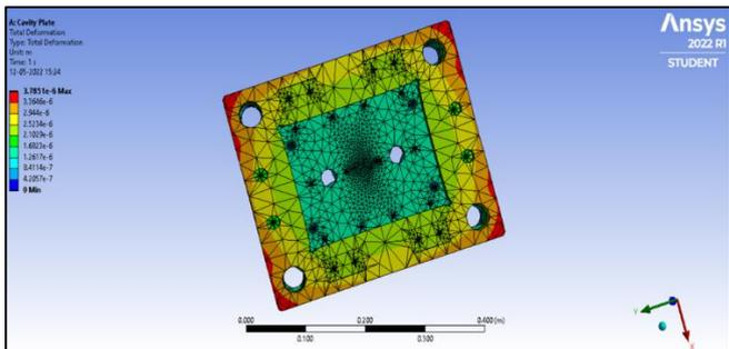
Figure 47: Total deformation of Cavity Housing
