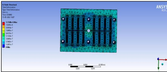
Figure 39: Total deformation of Cavity Block
