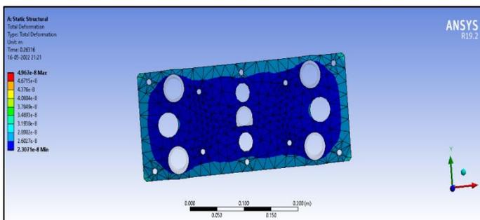
Figure 42: Total deformation of Ejector Back Plate
