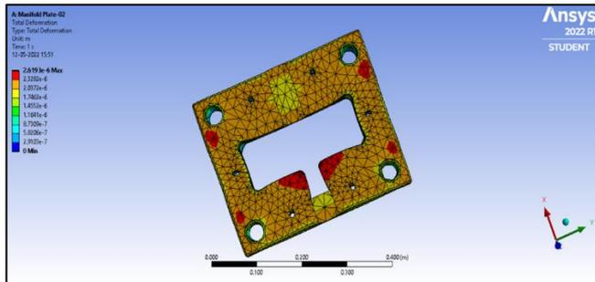
Figure 50: Total deformation of Manifold Plate
