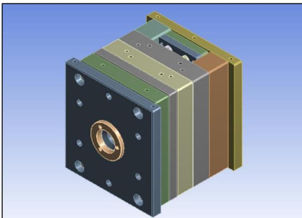
Figure 34: Assembly of Mold
