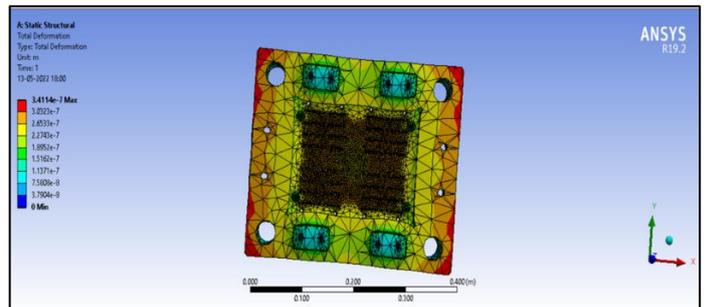
Figure 36: Total deformation of Core Housing
