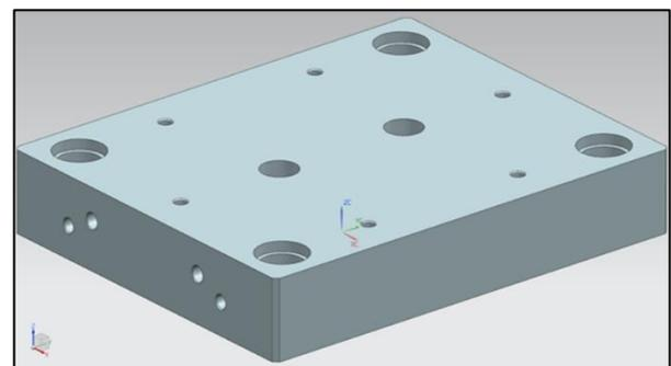
Figure 16: Cavity Housing Bottom view
