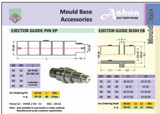
Figure 9: Standard size for Ejector Guide Pin and Ejector Guide Bush
