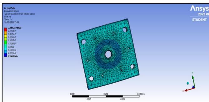
Figure 53: Stresses induced in Top Plate
