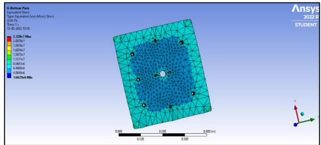
Figure 45: Stress induced in Bottom Plate
