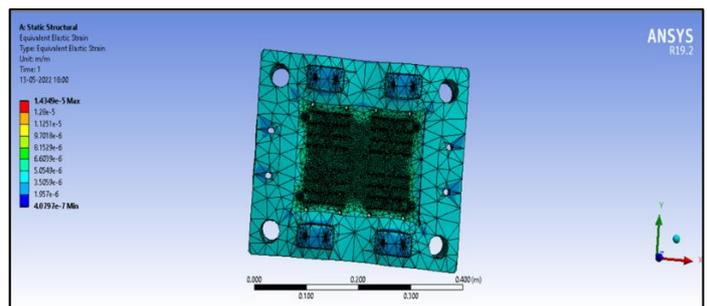
Figure 37: Stress induced in Core Housing
