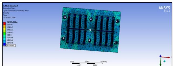
Figure 38: Stress induced in Cavity Block
