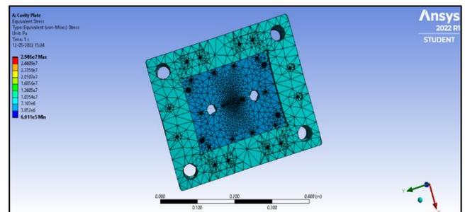
Figure 48: Stress induced in Cavity Housing
