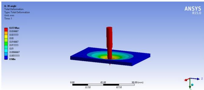
Fig-9- Deformation at 30<sup>0</sup> Tool
