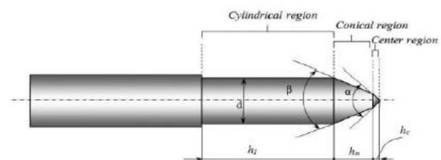
Fig-2: Shape of Friction Drilling Tool
