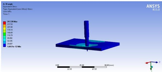
Fig-10- Equivalent Stress at 30<sup>0</sup> Tool
