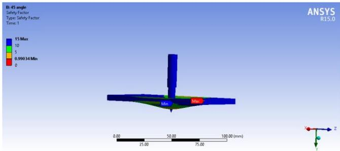
Fig-8- Safety Factor of 45<sup>0</sup> Tool
