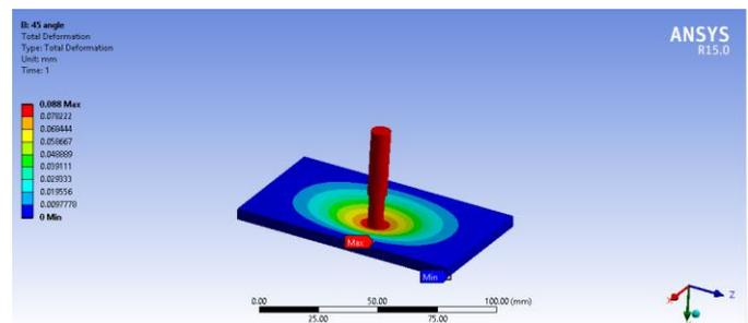
Fig-7- Deformation of 45° Tool
