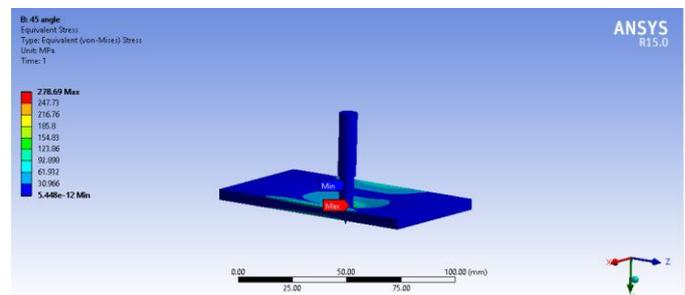
Fig-8- Equivalent Stress of 45° Tool
