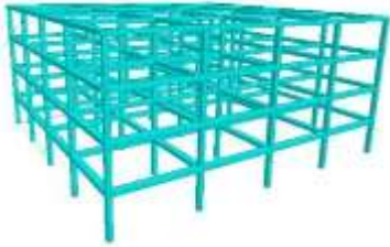
FIG 4: 3d Rendered model after specifying the properties to member.
