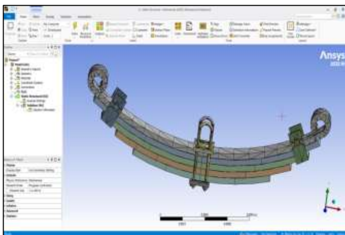
Fig- 4: Generating Mesh on Model
