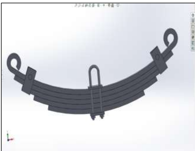
Fig- 2: Assembly of Leaf Spring
