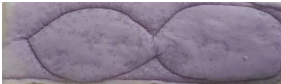
Fig 5.12: F (Non-treated lotus stem fibre) sanitary napkin after absorption of fluid
