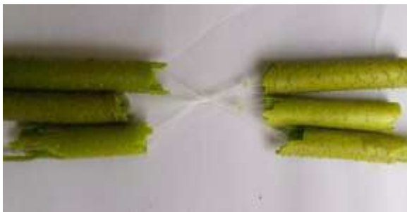
(c) separating the fibers from the stems
