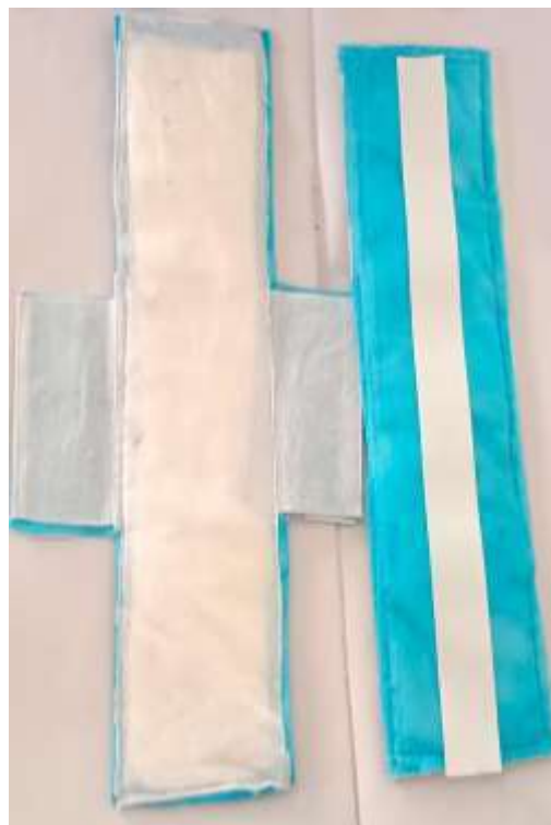
Figure 4.5: Front and back side napkin by using Lotus stem fibre
