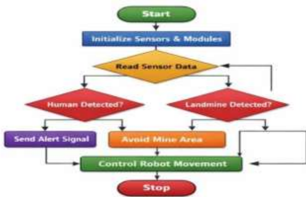
Fig 1: Block diagram of the spyder bot.
